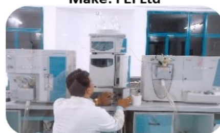
Liquid Chromatography-with Mass Spectrometry Model: LCQ Fleet and TSQ Quantum, Make: Thermo Scientific
